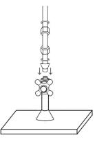
4. On the opposite end of the supply line, take a rubber cone washer and place it on the supply line with the flat side against the lip in the lines. Slide the slip nut and friction washer that you put on the pipe in step 3, up to the top of the lines. Tighten the nut to the faucet through the moutning holes of the tub.
