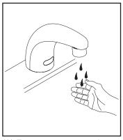
(9) Factory preset sensing distance is 12 cm (~4.7 in), please place an object or hand at about this distance and let water flush any debris from supply line for at leas one minute. Put aerator back to spout and press ON/ OFF button again.
