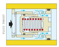
If the differential pressure is within the control range, the spring-loaded piston is positioned to give the fluid a free flow area permitting regular flow at the **nominal rate** for which the FlowCal™ is set up.
