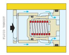
In this case, the spring-loaded piston fully compresses a spring and leaves only the fixed orifice for the fluid to pass through.
