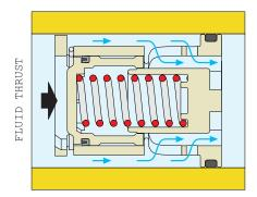
In this case, the spring-loaded regulating piston remains in equilibrium without compressing the spring and gives the fluid the maximum free flow area. When below the differential pressure control range the piston acts as a fixed orifice and thus the flow rate through the FlowCal™ depends only on the differential pressure.
