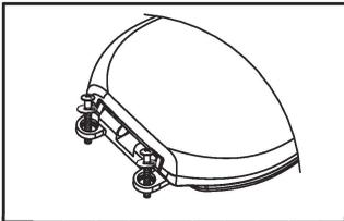
2. Insert the washers and bolts into the toilet seat installation holes.
