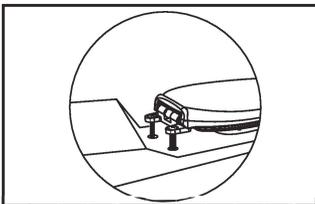
3. Check the fit of the toilet seat to the rim of the toilet bowl. Adjust the position of the seat if necessary.
