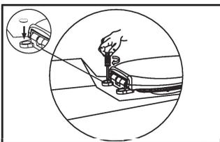
4. Tighten the bolts until the seat is securely attached. Install the plastic caps to cover the bolts.
