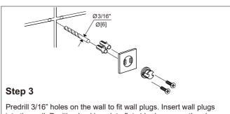
Predrill 3/16" holes on the wall to fit wall plugs. Insert wall plugs into the wall. Position backing plate flat side down over the plugs and install screws.
