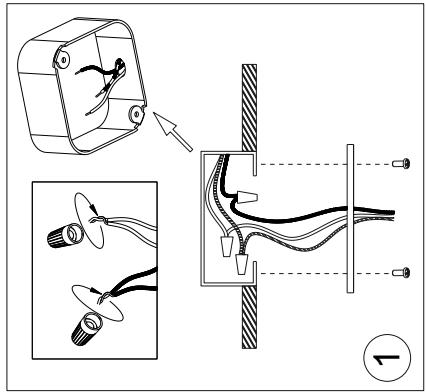
Fasten open end of ground wire (bare copper or green wire) to ground wire or ground screw of junction box, or ground screw on back plate. Connect black wire of power supply to black wire of fixture, and white wire of power supply to white wire of fixture using wire connectors.
