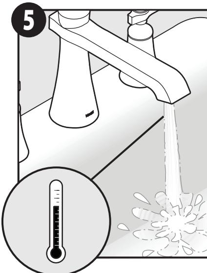
Minimum flow rate= 1.0gpm (3.8L/min)
