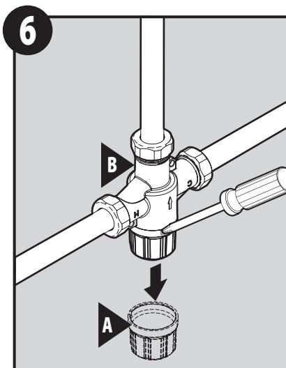
To adjust temperature: Align triangle on top of Adjustment Cap (A) with triangle on top of Valve Body (B). Twist counter clockwise for hot or clockwise for cold.
