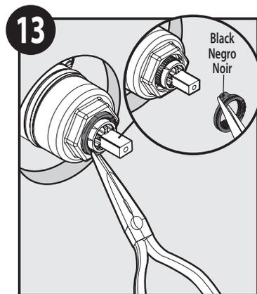
Remove the adjustable temperature limit stop.
