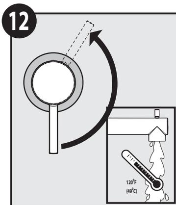
Rotate the lever until the water is to the maximum desired temperature, not to exceed 120°F (49°C). Seasonal maintenance of the maximum outlet temperature may be required due to changes in groundwater temperature.
