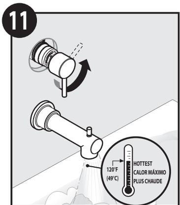
Open handle to full hot to test hot water temperature. Close handle if desired water temperature has been met. Hot water temperature should not exceed 120°F.
