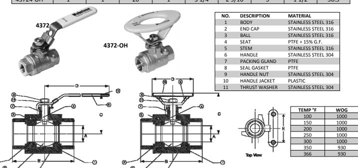
**Specifications:** Designed for residential, commercial or industrial use with water, oil or gas. This approved Webstone valve is actuated by a blowout proof stem and features an adjustable packing gland. It features an actuator mount, ideal for use in applications where automating the valve's operation is desired (actuator not included). Threaded ends comply with ANSI B1.20.1.
