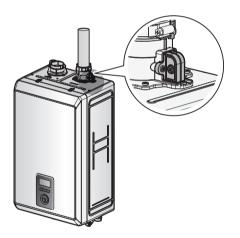
As shown, the VID is a device connected to the vent collar which is intended to detect whether the vent pipe has been inserted to a sufficient depth into the collar during its initial installation.
