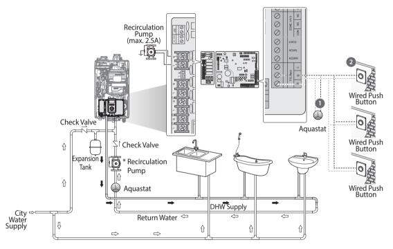
\* A Taco 008-BC6 or Grundfos 15-42 BUC7 (or equivalent) circulation pump is recommended for use with the NCB-H boiler and DHW recirculation systems.
