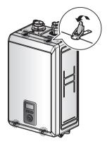
9. Loosen the screws indicated in the figure below and connect a manometer to the pressure port. Reset the manometer to zero before use.
