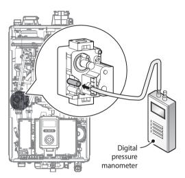
Figure 9. Connect Digital Pressure Monometer
