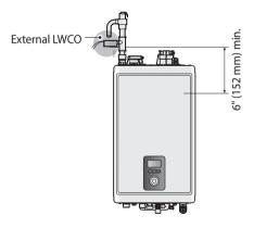
Figure 1. External LWCO (without Navien Manifold System)
