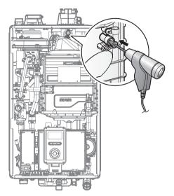
Figure 7. Insert the Analyzer
