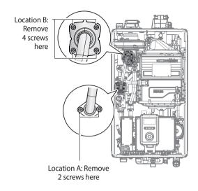
Figure 3. Detaching Gas Valve from Gas Inlet Pipe and Fan Motor Assembly
