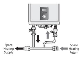
Note Refer to the following illustration for details on installing the NCB-H Manifold System (Part Number: 30026576A) to the valve kits.
