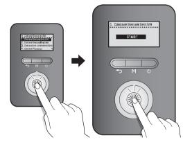
3. On the sub NPE-A2 water heater panel, press and hold the OK button (OK) for 3 seconds on the sub unit. Then, the **ID 1. Allocated!** message will appear on the sub unit's front panel display. When the water heater is set to a sub unit, the **S** icon will appear on the display.
