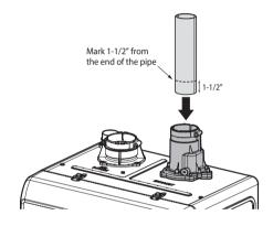
2. Insert the vent pipe into the vent collar to start the vent run. Make sure to completely slide the vent into the collar until the end makes contact with the bottom of the socket.
