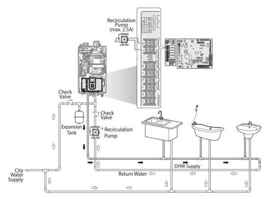
\* A Taco 008-BC6 or Grundfos 15-42 BUC7 (or equivalent) circulation pump is recommended for use with the NCB-H boiler and DHW recirculation systems.
