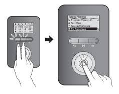
Rotate the Command dial ( to switch between the parameters. Press the Command dial ( to run an air purge.
