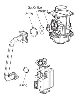
Figure 5. Exploded View of Gas Pipe Assembly
