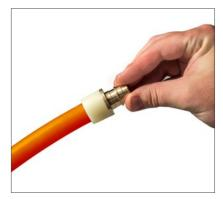
4. Insert fitting into expanded tube and sleeve. Assure proper expansion so that fitting is touching tube and sleeve. Hold fitting in place until tube/sleeve memory constrict annularly around the fitting.
