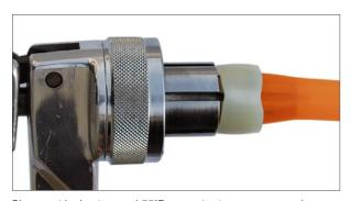
Ring must be kept around 55°F or greater to assure expansion is uniform. Remove any expanded ring that displays unequal expansion.
