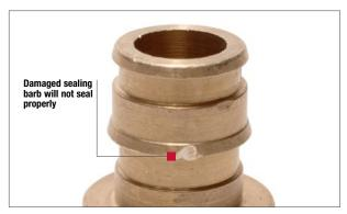
Damaged, cut or grooved sealing barb.
